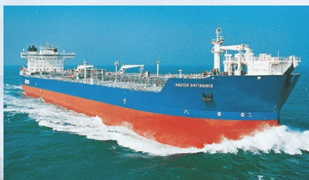
Shuttle Tanker «Navion Brittania» is equipped with 2x2200 kW Retractable Tunnel Thrusters in bow, 1x1400 kW Retractable Tunnel Thruster in stern. (1998)
