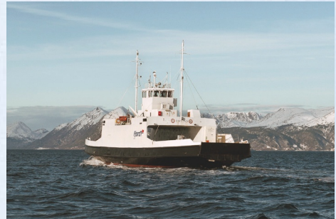
The ferry "Eiksund" have 2x380kW Azimuth Propulsion RDT.
