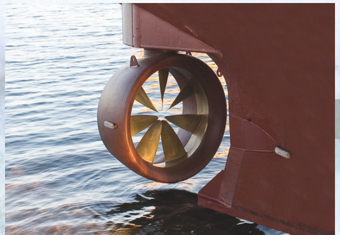
One of the Azimuthing RDTs installed in the ferry "Eiksund"
