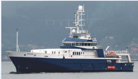
Fishing Research Vessel "Nordsøen" have a 300kW RDT in bow and a 160kW RDT in stern.
