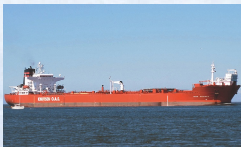
«Tove Knutsen» was the first Shuttle Tanker in the world to be equipped with a Brunvoll Retractable Combi Azimuth/Tunnel Thruster - 2000 kW forward. (2004)
