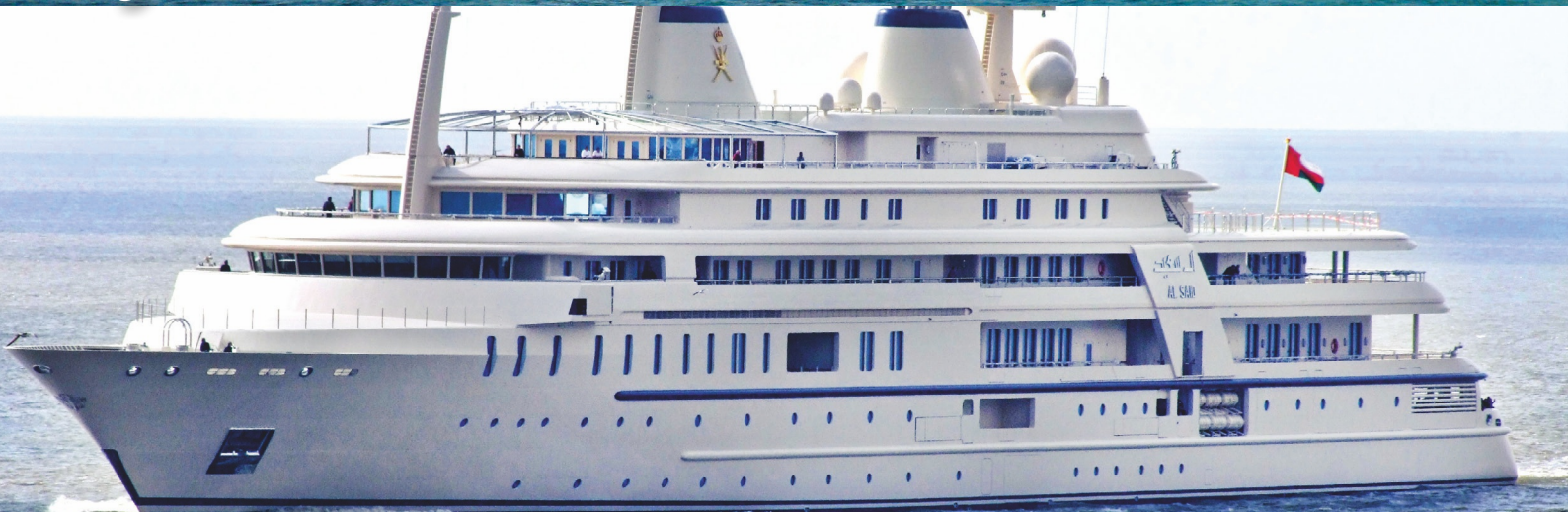
4 2008 "Al Said" (155m) has six spacious decks. Shrouded in secrecy, the yacht has a concert room with space for a 50-piece orchestra. Bow: 2 x LowNoise FU63 LRC 1750 550 kW. Stern: 2 x FU37 LRC 1000 200 kW.
